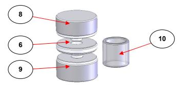
Fig 2. 7mm Pellet Die Assembly Complete
